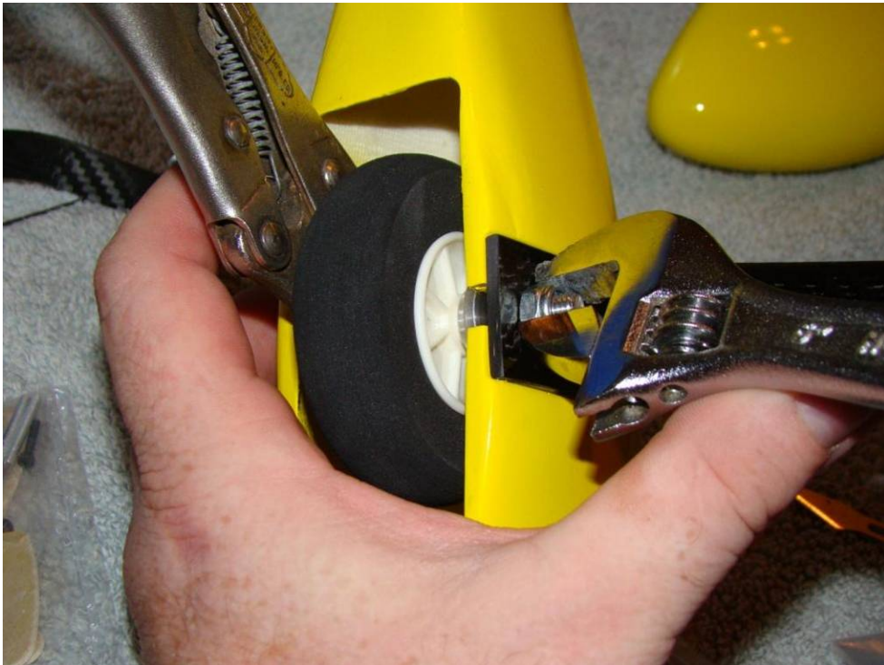
Slide one wheel/axle assembly into a wheel pant, and install the wheel assembly on the landing gear leg. Tighten the locknut as shown to secure the assembly onto the gear leg. Repeat for other side.
