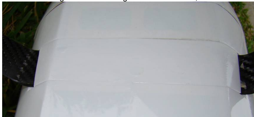
Install gear cover plate as shown, using thick CA or epoxy glue.
