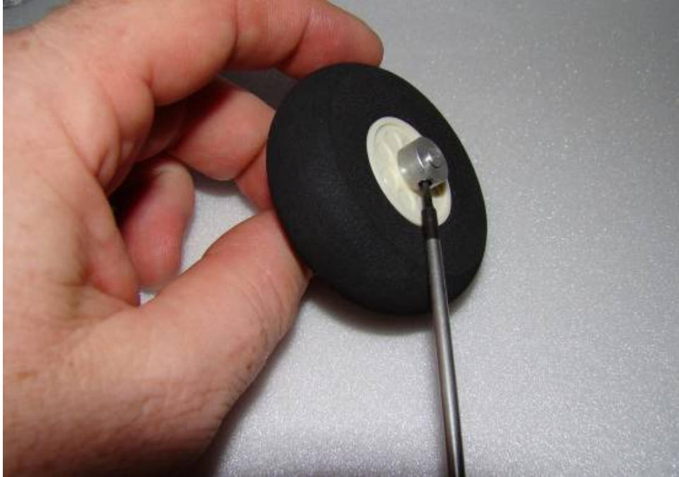
Install the wheels onto the axles and secure with the wheel collars, as shown.
