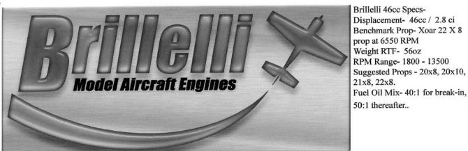
Brillelli 46cc Specs-Displacement- 46cc / 2.8 ci Benchmark Prop- Xoar 22 X 8 prop at 6550 RPM Weight RTF- 56oz RPM Range- 1800 - 13500 Suggested Props - 20x8, 20x10, 21x8, 22x8.
